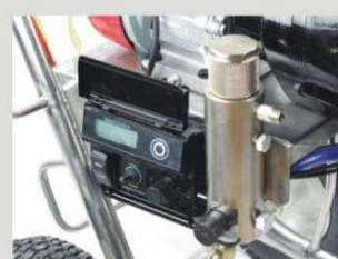
EZ pressure control system delivers a consistent spray fan without pressure fluctuations at all spraying pressures.
